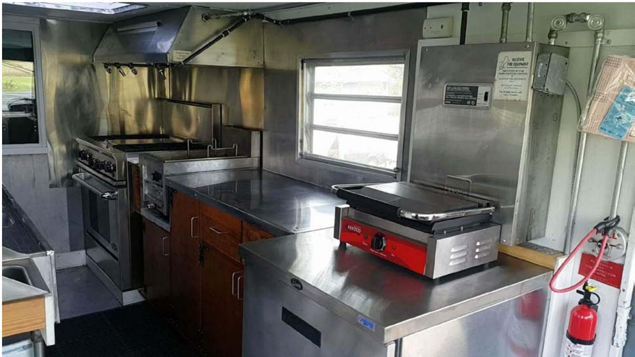
Figure 4: General layout of the truck, including oven, stove, cabinet, frier, serving window, and panini press.
